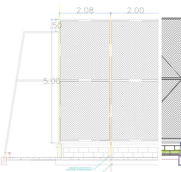
DETALLE ARQ. DE COLUMNETAS ESC1:40
