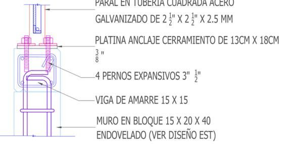
DETALLE ANCLAJE CERRAMIENTO ESCALA 1:5
